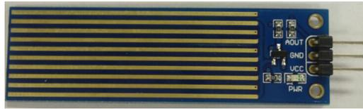
Gambar 3.2: Hardware sensor Liquid Level
